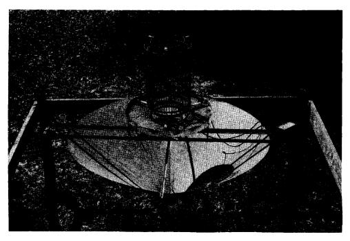
Fig. 1. Sound trap, including electrocution grid, plywood ring, sound synthesizer (protective plastic bag just visible through hole in ring), sheet-metal funnel, and catching jar. Funnel, ring, and synthesizer are supported by a steel yoke attached at either end to posts 1.3 m tall.
