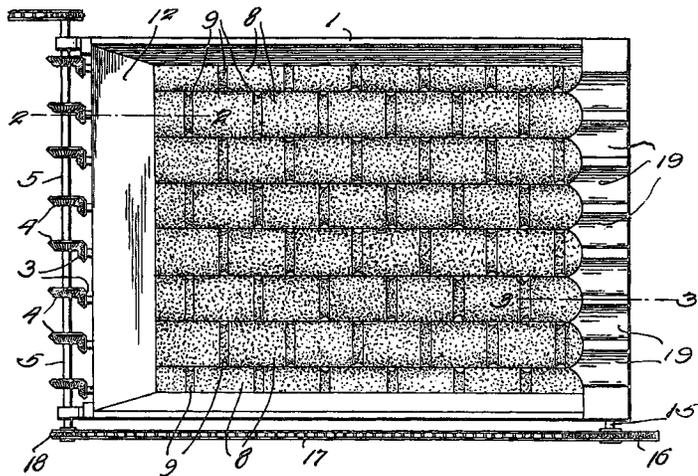
Fig. 2. Lateral brusher. Fruit travels along brush grooves from left to right. Often sloped downhill to encourage fruit movement (From US Patent 1,417,266).
