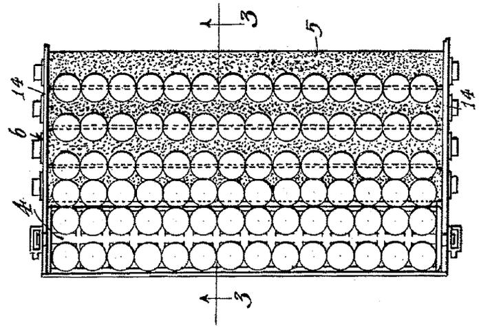
Fig. 3. Transverse brusher. Fruit movement is from bottom to top. Fruit moves by pressure from incoming fruit and rotation of brushes. Entire top surface of brush comes into use (From US Patent 1,970,861).
